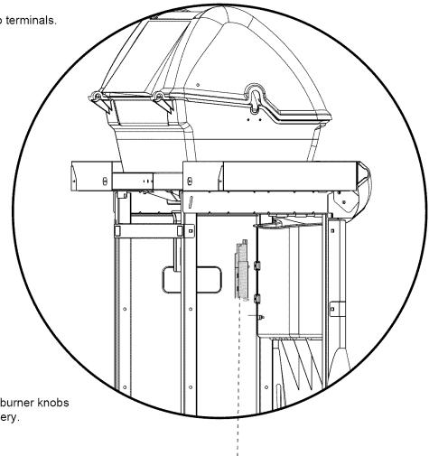
33. After wiring ignitor module ensure that all burner knobs are in the off position **before** installing the battery.
